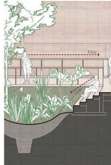
Integrated between the built spaces, the bioswales not only manage stormwater but also create spaces for seating and leisure.
